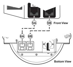
Figure 2-8 — Configuration of RJ-45 connectors
